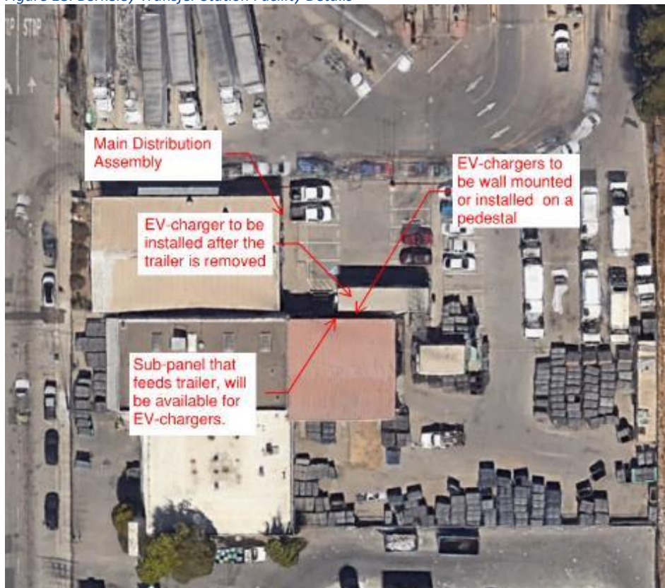
Figure 18: Berkeley Transfer Station Facility Details
